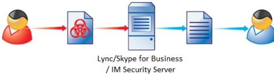
**FIGURE 1-2. How IM Security Virus Scan works**
